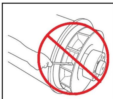
FIGURE 18. DO NOT ROTATE THE ALTERNATOR ROTOR WITH A LEVER
