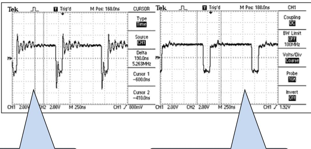
Trace from a network with excess stub length
