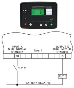
In case of set 1 failure, the output activates and energizes the external relay RLY1 to call for the second set to start.
