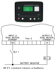
RLY1 contact closes a battery negative signal onto the input, instructing the set to start.
