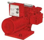
Efficient, High Performance, Light enough for portable application. Alternator: Rotating armature, 2 pole, static excitation, ± 5% voltage regulation. Engine: 5 H.P. Briggs & Stratton, 4-cycle, recoil starter, heavy duty rear main ball bearing. Standard Equipment: Fuel Tank, Muffler, Vibration Isolators, Receptacles, Econ-O-Mizer Idler Control
