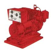
Rugged, compact, Portable Power, ideal for contractors, rental yards, low cost standby. Alternator: Rotating field, 2 pole, static excitation, 5% voltage regulation, Total Power and load control. Engine: 81/4 H.P. Wisconsin, 4 cycle, recoil starter, heavy duty tapered roller bearings, valve rotators. Standard Equipment: Fuel Tank, Muffler, Vibration Isolators, Receptacles.
