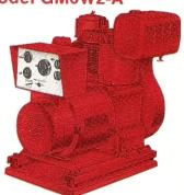
More watts per pound - designed to operate the larger motors on construction tools. Alternator: Rotating field, 2 pole, static excitation, 5% voltage regulation, Total Power and load control. Engine: 12.5 H.P. Wisconsin, 4 cycle, rope start, heavy duty tapered roller bearings, valve rotators. Standard Equipment: Fuel Tank, Muffler, Vibration Isolators, Receptacles.
