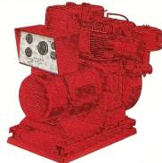
Dependable - Rugged - Compact. Alternator: Rotating field, 2 pole, static excitation, 5% voltage regulation, drip-proof construction. Engine: 10 H.P. cast iron, 4 cycle, single cylinder engine, Briggs & Stratton. Standard Equipment: Fuel Tank, Muffler, Vibration Isolators, Receptacles, Recoil Starter, Econ-O-Mizer Idler Control.
