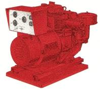
Rugged, compact, Portable Power, ideal for contractors, rental yards and low cost standby. Alternator: Rotating field, 2 pole, static excitation, 5% voltage regulation, total power and load control. Engine: 8 H.P. Briggs & Stratton 4 cycle, recoil starter, heavy duty ball bearings. Standard Equipment: Fuel Tank, Muffler, Vibration Isolators, Receptacles, Econ-O-Mizer Idler Control.
