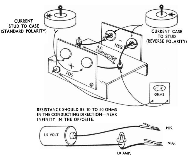
ALTERNATE MEANS FOR TESTING A DIODE IF AN OHMMETER IS NOT AVAILABLE. NOTE: TO CHECK CONDUCTING DIRECTION CONNECT POSITIVE AT BASE OF ARROW AND NEGATIVE AT POINT. EXAMPLE: STUD ON STANDARD; CASE ON REVERSE.
