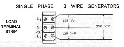
Two circuits, of ½ generator capacity each, are available at 125 volts. Load can be combination of 250 volts and 125 volts. Care must be used not to overload either line. Subtract the 250 volt current from the nameplate amperes. The difference is available at 125 volts on each line. Excessive overload on any or all lines will trip the load breaker.
