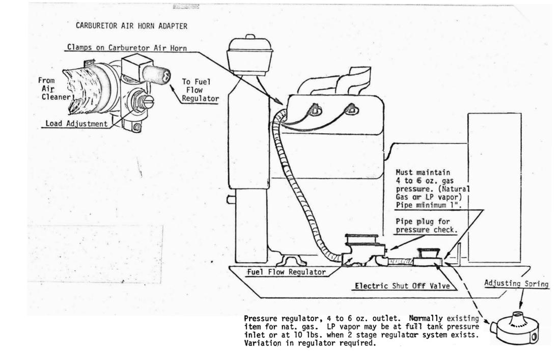
15 KW-WISCONSIN VG4D NATURAL GAS OR VAPOR WITHDRAWAL LIQUEFIED PETROLEUM
