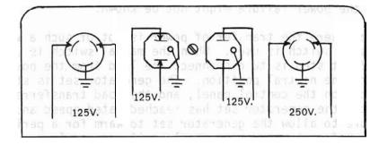
Twistlock receptacles are convenient for power cord with terminal box end (can't be accidently disconnected). Duplex outlet can be used for similtaneous adjacent power within generator capacity limits. Combination load at 125 volts and 250 volts is available. Example: 20 areas at 125 volts = 2500 watts
