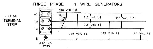
Three phase  $(3\phi)$  generators can be used for  $3\phi$  load at 216 volts nominal and also single phase load at both 216 volts and 125 volts. The total current in any line should be the sum of both single and three phase as listed on the nameplate amps, per terminal. Single phase load should be distributed as evenly as possible to avoid overloading any one line. Example: nameplate amps, per term, -40
