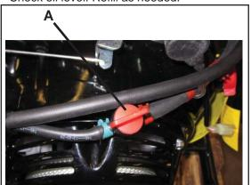
2. Turn on the fuel supply by moving the fuel lever to the position shown.
