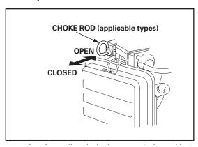
Move the choke lever to the "CLOSED" position.
