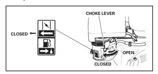
3. Move the choke lever to the "CLOSED" position. To restart a warm engine, leave the choke lever in the "OPEN" position
