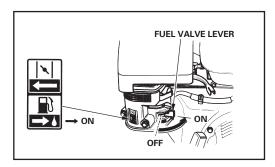
2. Turn on the fuel supply by moving the fuel lever to the "ON" position.
