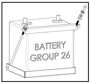
You will need to purchase and install a battery to operate this engine generator set. A twelve volt battery, group 26 rated at 500 CCA or larger is recommended for this electric start engine generator set. Follow the battery manufacturer's recommendations for servicing and charging prior to use. Connect the battery to the electric start system using the cables provided.
