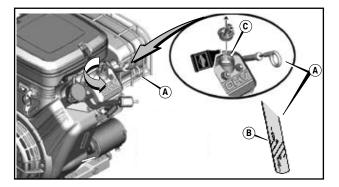
Oil is added to the engine by removing the oil fill cap (ref "C") and adding oil at this point. After filling the crankcase to the proper level, be sure you properly tighten the oil fill cap. NOTE: This engine generator must be on a level surface before you check or add oil to the system.
