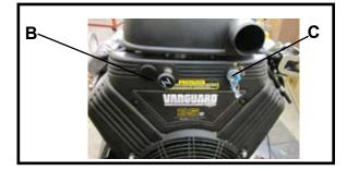
3. Move the choke to the full "on" position. A warm engine will require less choking than a cold engine. Ref "B"
