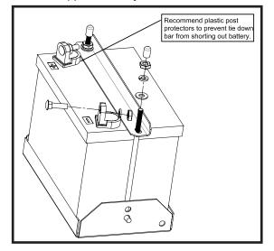
If you intend to use the power plant's electric start system, you will need to purchase and install a battery to operate it. Units equipped with a recoil or rope start will operate satisfactorily without a battery.
