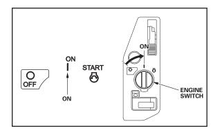
5.. Operating the starter. Rotate the key switch briefly to the START position. The starter life is improved by using shorter starting cycles with time to cool off between cranking cycles. Do not operate the starter more than 5 seconds and wait at least 10 seconds before operating the starter again, Repeat cycle if necessary.
