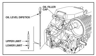
Oil is added to the engine by removing the oil fill cap and adding oil at this point. After filling the crankcase to the proper level, be sure you properly tighten the oil fill cap. NOTE: This engine generator must be on a level surface before you check or add oil to the system.
