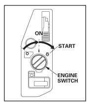
6. When the engine starts, release the key switch, allowing it to return to the "on" position.
