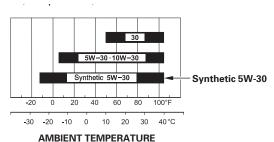
SAE 10W-30 or 5W-30 is recommended for general use. Use a full synthetic 5W-30 for starting/operating temperatures between 5°F (-15°C) and -13°F (-25°C). Other viscosities shown in the chart may be used when the average temperature in your area is within the indicated range.
