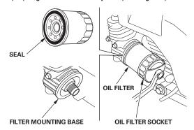
**NOTE:** This engine requires 57 to 58 ounces (1.78 to 1.81 quarts) of oil if it is completely drained. Use caution when refilling the engine as some residual oil may have remained in the engine. Always use the dipstick when filling the engine with oil to prevent overfilling.
