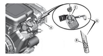
Oil is added to the engine by removing the oil cap and adding oil at this point. After filling the crankcase to the proper level, be sure you properly tighten the oil fill cap ('C').
