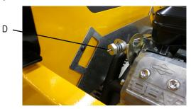
CAUTION: EQUIPMENT DAMAGE SPEED ADJUSTMENTS SHOULD ONLY BE MADE BY A QUALIFIED SERVICE TECH. Whenever making any speed adjustments, check the unit with a voltmeter and a frequency meter or a tachometer and be sure the voltage and speed are correct.
