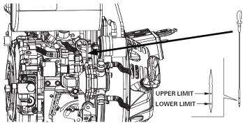
Oil is added to the engine by removing the oil cap and adding oil at this point. After filling the crankcase to the proper level, be sure you properly tighten the oil fill cap.
