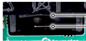
Install Battery Between These Two Points
