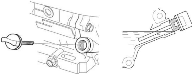
Oil is added to the engine by removing the oil cap and adding oil at this point. After filling the crankcase to the proper level, be sure you properly tighten the oil fill cap.
