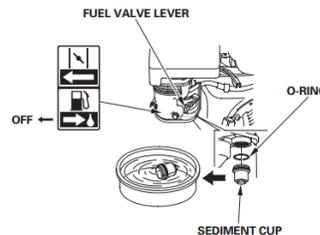
3. Place the O-Ring in the fuel valve and install the sediment cup. Tighten the sediment cup securely.
