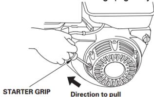
Note: Do not allow the starter grip to snap back against the engine. Return it gently to prevent damage to the starter.
