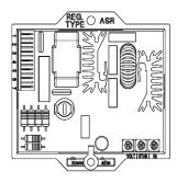
The following is a list of connections on the AVR. These have been factory set and other than voltage adjustment, should never be changed.
