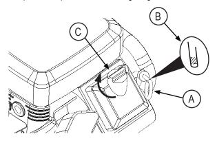
If needed, oil is added to the engine by removing the oil cap and adding oil at this point. After filling the crankcase to the proper level, be sure you properly tighten the oil fill cap ('C').
