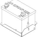
If you intend to use the unit's electric start system, you will need to purchase and install a battery to operate it. A 12 Volt battery, BCI group 26 rated at 500 CCA or larger is recommended for this electric start engine-generator set. Follow the battery manufacturers recommendations for servicing and charging prior to use. Connect the battery to the electric start system using the cables provided.
