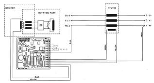
VOLT: Voltage. Rotate clockwise to increase voltage. STAB: Stability. HZ: Low Frequency. AMP: Overload.
