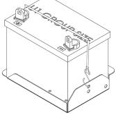
A customer supplied 12 Volt battery, BCI group U1 rated at 300 CCA or larger is recommended for this electric start engine-generator set. Follow the battery manufacturers recommendations for servicing and charging prior to use. Connect the battery to the electric start system using the cables provided.
