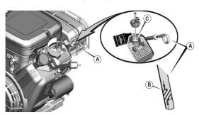
Oil is added to the engine by removing the oil cap (ref. 'C') and adding oil at this point. After filling the crankcase to the proper level, be sure you properly tighten the oil fill cap.
