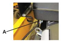
3. Engage the choke by pulling it out. A warm engine will require less choking than a cold engine.
