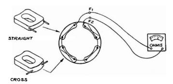
**NOTE:** Fields alternate "straight" and "crossed" to provide proper polarity. When ordering replacement coils be sure to include Model, Type, and Serial Number.
