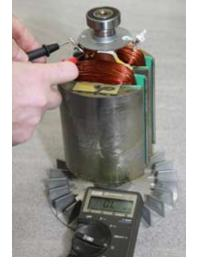
4. Check rotor leads for continuity and grounding. Place meter leads on solder end of diode(s). At least one of the diodes must be disconnected from the rotor to check continuity and resistance. There should be continuity between the leads and no reading to ground (metal shaft). The expected resistance values are listed in the table at the end of this guide. If rotor is out of specification or is grounded replace the rotor.
