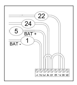
The following is an optional way to interconnect the Generator and the Transfer Switch. The wires terminate on TB7 as follows:
