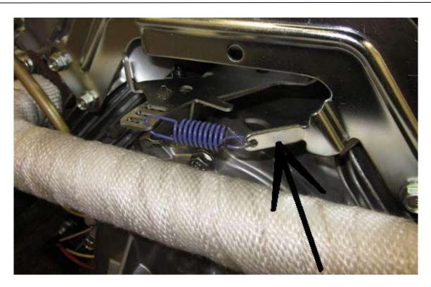
BEND THIS TAB TO CHANGE THE ENGINE SPEED (FREQUENCY). STRETCHING SPRING INCREASES THE FREQUENCY (INCREASES ENGINE SPEED).
