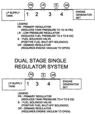
Reference numbers 1 through 3 in the block diagrams above are system parts supplied by customer.
