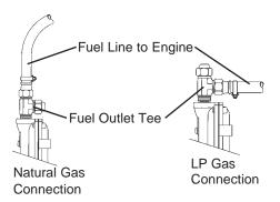
If you are going to operate on LPG you will need to move the fuel line from the NG port to the LPG port on the fuel outlet tee. These two ports have different orifice inserts installed in them, which provide proper engine operation with no further adjustments.
