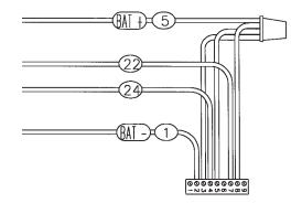
The following is an optional way to interconnect the Generator and the Transfer Switch. The wires terminate on TB7 as follows:
