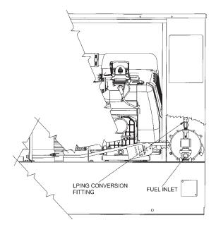
column). These fuel pressures are critical; failure to provide the proper fuel pressure can cause many problems ranging from a unit that will not start to causing damage to the fuel system.
