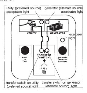
4. Press and hold the **Push to Test** button until the generator (alternate source) acceptable light comes on and stays on. Then release the button. This will start up your generator set.
