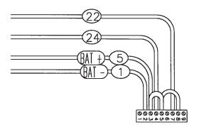
The following is an optional way to interconnect the Generator and the Transfer Switch. The wires terminate on TB7 as follows:
