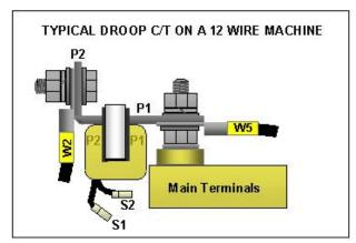
The most important aspect of initial setting up procedure concerns the droop circuit. Most of the troubles allied to poor load sharing originate from the droop circuit. They are either incorrectly adjusted for the level of voltage droop, or are incorrectly connected, (reverse droop), such that a rising voltage characteristic is obtained.
