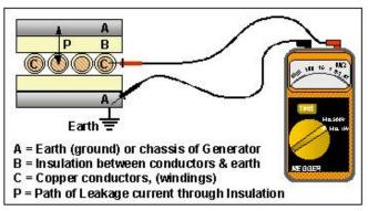
The high voltage causes a current to 'leak' through the insulation system. This current produces an output reading on the Insulation tester ('Megger'), which is measured in Megohms (resistance to earth or ground). A normal value for a low voltage Generator winding should be higher than 1 Megohm to earth.
