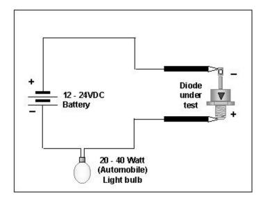
A good diode will light the bulb in only one direction. It should not light when test leads are reversed on the diode pin and base.
