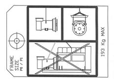
Warning: The generator lifting points are designed to lift the generator only. Do not lift the complete generating set by the generator lifting lugs.
