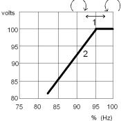
Clockwise adjustment lowers the frequency (speed) setting of the "knee point" and extinguishes the LED. For Optimum setting the LED should illuminate as the frequency falls just below remind frequency i.e. 47Hz on a 50Hz generator or 57Hz on a 60Hz generator.
