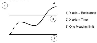
The illustration shows a typical curve for a machine that has absorbed a considerable amount of moisture. The curve indicates a temporary increase in resistance, a fall and then a gradual rise to a steady state. Point 'A', the steady state, must be greater than 1.0 Megohm (If the windings are only slightly damp the dotted portion of the curve may not appear).
