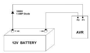
Caution! If the generating set battery is used for field flashing, the generator main stator neutral must be disconnected from earth.
