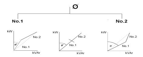
Generally 5% droop at full load current zero p.f. is sufficient to ensure kVAr sharing.
