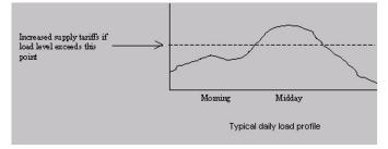
In some cases, it can be more cost effective for the customer to provide an alternative power supply during this time of higher tariff. There are a number of possibilities open to the customer:
