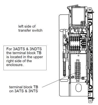
Engine start and auxiliary circuit terminal block TB located on 3ATS &3NTS transfer switch.
