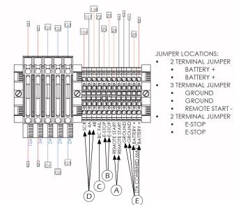
A - Customer Remote Start CONNECTIONS TERMINALS. The two remote start leads from the Automatic Transfer Switch are connected to the two terminals marked Remote Start and Remote Start. The wire in terminal labeled #1 is Battery Negative/Ground and the wire in the terminal labeled #23 is your Remote Start lead. Closing these two leads together will signal the DSE 7310 MKII to go into an autostart mode and start up the engine generator.
