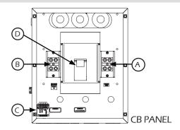
A - Neutral Lugs, These neutral lugs are isolated from ground and provided for you to connect your neutral wire from the transfer switch. The lugs will handle wire sizes #1 AWG TO 300 MCM and should be torqued to 250 in. lbs.
