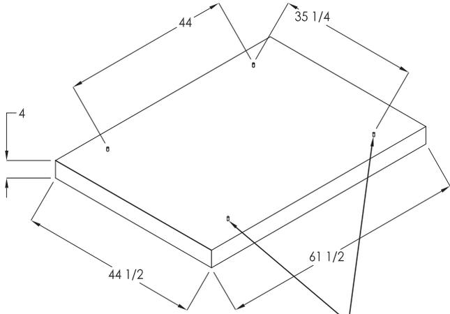
CONDUIT CONNECTION POINTS ON SIDE OF GENERATOR CABINET AND FRAME.
