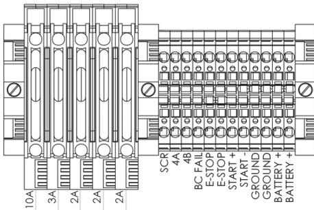
The E-Stop and Remote Start wires have been wired from the controller terminals to the panel for easy installation.
