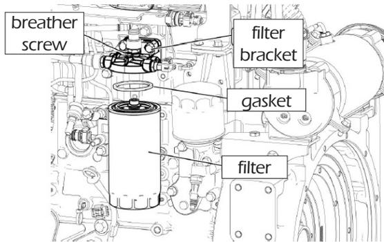
1. Remove the filter by unscrewing it. Keep gasket.
