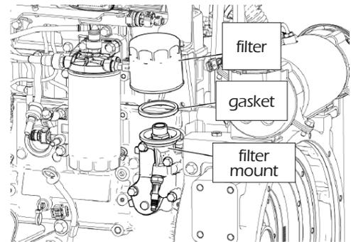
The filter must be replaced when the lubricant oil is changed.
