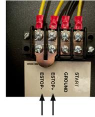
In some applications additional emergency stops may be desired or necessary. The controller has terminals designed allowing the addition of multiple remote emergency stops. E-stops must be normally closed to work properly in this system. The e-stop circuit supplies power to the fuel solenoid and the starter circuit. Opening any switch in the series prevents the engine from cranking or from receiving fuel to run.
