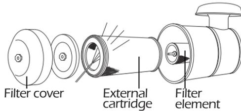
1. Remove the filter cover after first unscrewing the locking handle.
