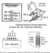
Your DC connection points in the ASCO 300 ATS are terminals "14" and "15". Depending on the size of the switch they are located in different locations.
