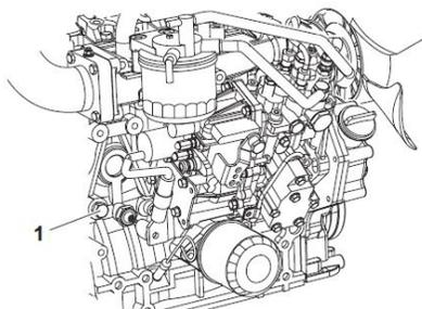
4. After draining the engine coolant, flush the radiator and engine block to remove any rust, scale and contaminants. Then reinstall and tighten the drain plug
