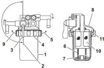
1. Position an approved container under the water separator (1) to collect the contaminants.
