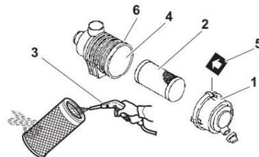
1. Unlatch and remove the air cleaner cover (1).
