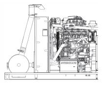
WINCO does not recommend that additional vibration isolators be installed between the generator base and the concrete pad. These can increase the total amount of vibration in the generator set causing component failures. Some applications and codes (example: Seismic) may require special vibration isolators. These items should be carefully engineered to ensure that the vibration when the generator set is operating normally is at a safe level and does not exceed component acceptable levels.
