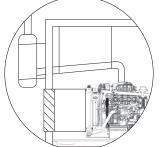
The muffler can be installed either inside or outside the shelter. Installing inside the shelter will increase the overall temperature and may require a larger shelter or additional air flow to prevent equipment overheating. In some cases, the muffler may require appropriate insulation to prevent radiant heat from affecting the equipment inside the shelter.
