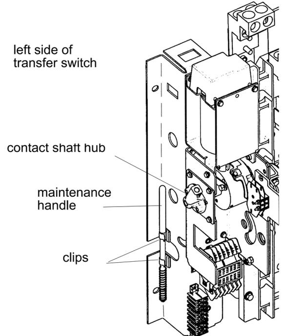
Figure 4. Maintenance handle on 3ATS & 3NTS.
