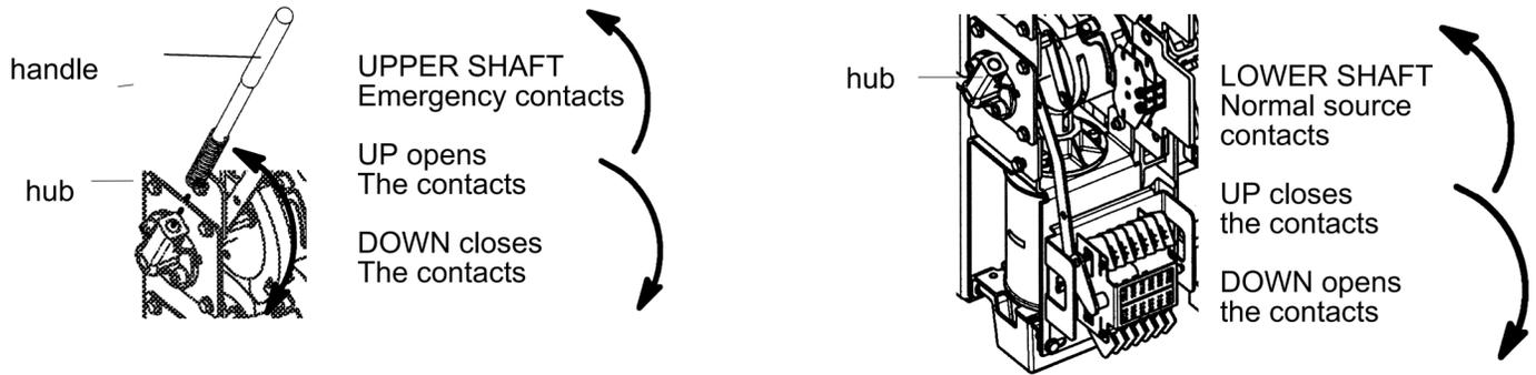
Figure 6. Maintenance handle operation on 3ADTS & 3NDTS
