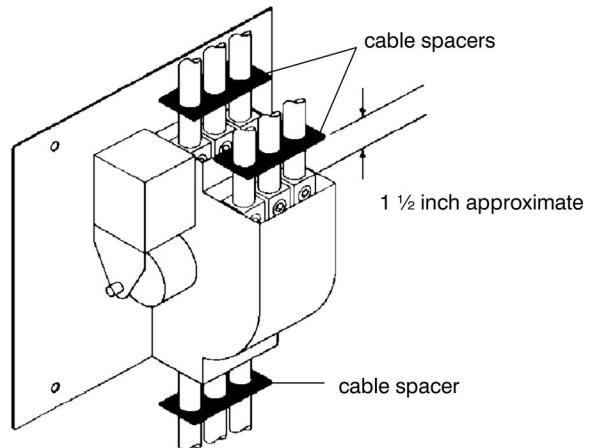
Figure 1-1. Cable spacers for 150, 200, and 230 ampere transfer switches.
