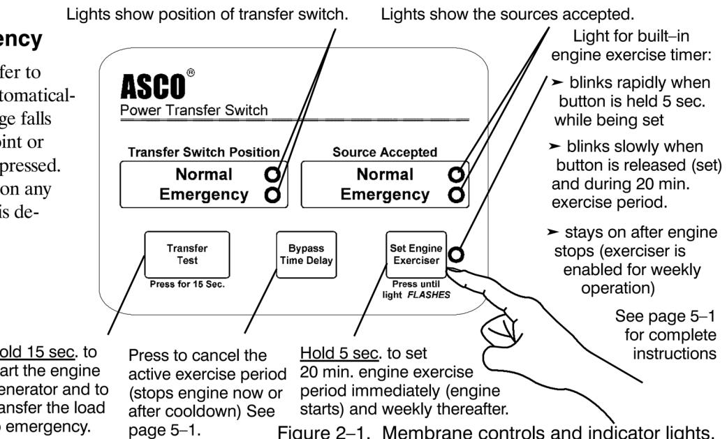
Figure 2-1. Membrane controls and indicator lights.
