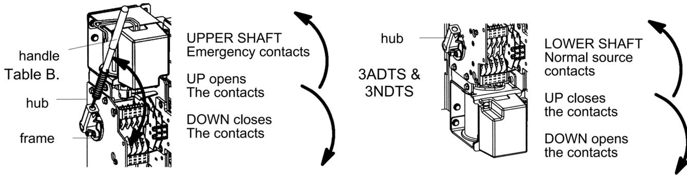
Figure 6. Maintenance handle operation on 3ADTS & 3NDTS
