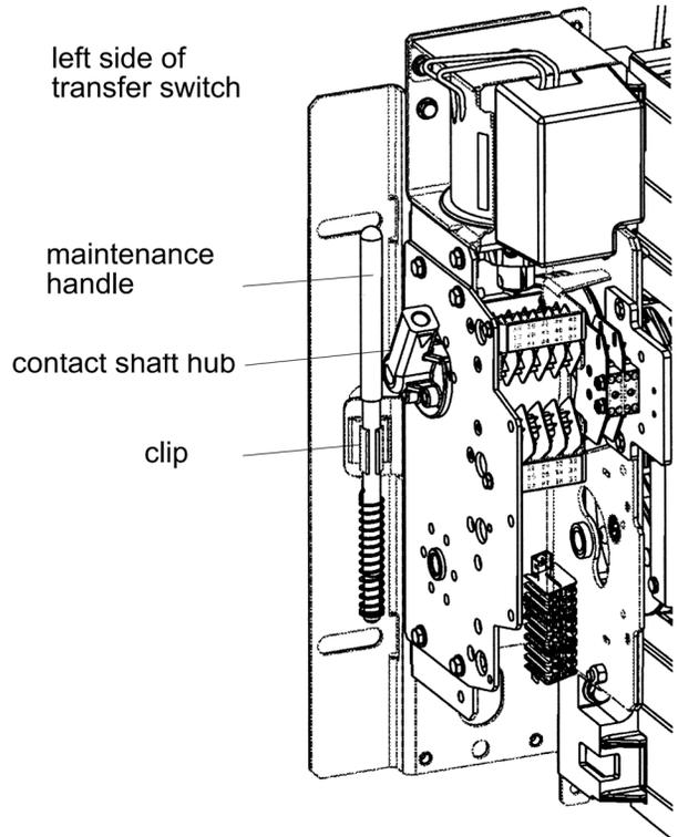
Figure 4. Maintenance handle on 3ATS & 3NTS
