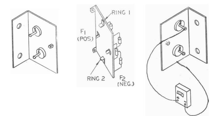
Note: Both diodes in each half of the control field bridge are pressed into the aluminum heat sink. Pressed in diodes require special tooling for replacement and cannot be changed in the field. Repair is made by replacement of assemblies.
