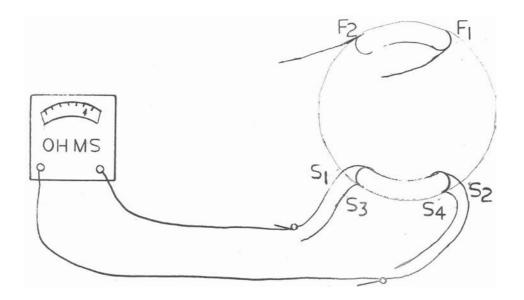
Note: The complete shunt field is wound in one coil and the series control field in the other.
