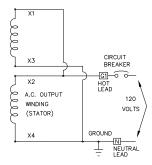
Check the appliance or tool nameplates for the current and voltage to ensure compatibility. Although a circuit breaker is provided, damage due to overloading constitutes abuse and will not be warranted. Refer to the generator nameplate for unit's capabilities.
