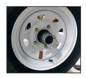
Pro Tip: Tighten lugs in a star pattern, until each lug is secure.
