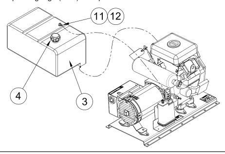
• Route customer supplied 1/4" fuel line from fuel tank to engine and attach the fuel line to the primer bulb (ref. 5) with red hose clamps. Attach 1/4" fuel hose (ref. 6) to the other side of the primer bulb (ref. 5) with red hose clamp (ref. 9) and route to the fuel filter (ref. A) on the engine. See step 5 below.
