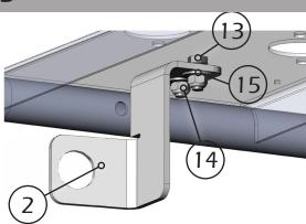
Next you will finish by installing the brake. Install the spindle (18) into the push pull toggle (4). Remove the large hex nut from the toggle. Install the toggle through the bracket (2) and the large hex nut. Secure the toggle to the bracket.
