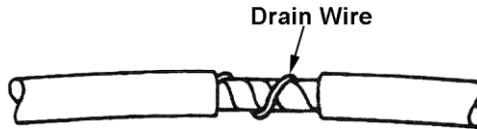
4. Splice wire using splice clips and rosin core solder. Wrap each splice to insulate.
