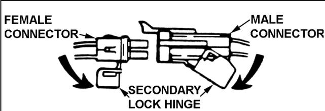
1. Open secondary lock hinge on connector.
