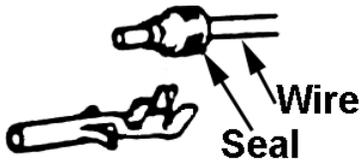
3. Cut wire immediately behind cable seal
