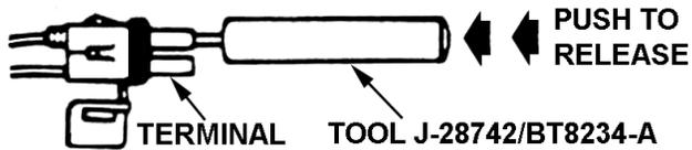
2. Remove terminal using tool.
