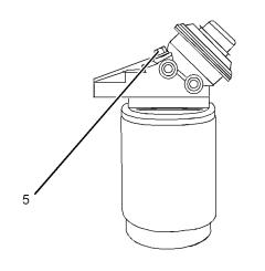
Illustration 52 Spin-on filter with fuel priming pump (5) Vent screw
