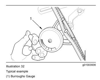
Install the gauge (1) at the center of the belt between the alternator and the crankshaft pulley and check the belt tension. The correct tension for a new belt is 400 N (90 lb) to 489 N (110 lb). The correct tension for a used belt that has been in operation for 30 minutes or more at the rated speed is 267 N (60 lb) to 356 N (80 lb).
