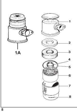
Never clean the filtering element  ${\bf 6}$  using solvents with a low flash point. This could cause an explosion !
