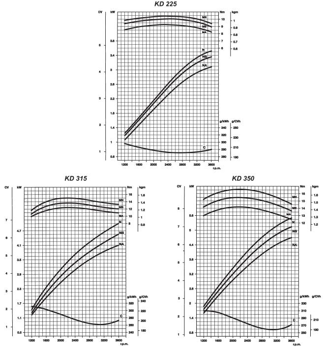
N (80/1269/EEC - ISO 1585) AUTOMOTIVE RATING : Intermittent operation with variable speed and variable load. NB (ISO 3046 - 1 IFN) RATING WITH NO OWERLOAD CAPABILITY: continuos ligth duty operation with constant speed and variable load. NA (ISO 3046 - 1 ICXN) CONTINUOS RATING WITH OVERLOAD CAPABILITY: continuos heavy duty with constant speed and constant load. NN Torque at N power.
