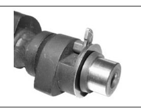
During normal operation, the tappet overcomes the spring resistance while passing on the system and decompression does not operate.
