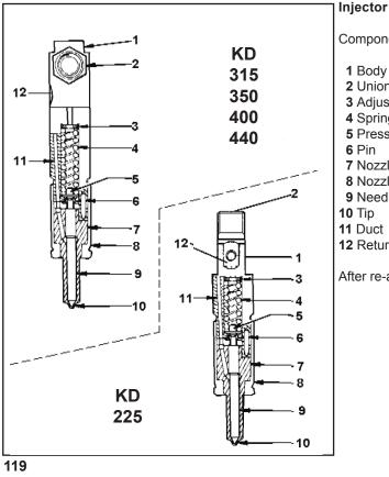
Components: 1 Body 2 Union 3 Adjusting shim 4 Spring
