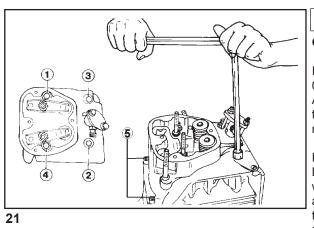
Do not demount when hot or the part could become deformed.
