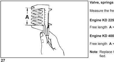
Measure the free length with a caliper.
