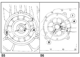
A warped oil retainer may allow the introduction of air into the engine thus causing crankcase ventilation problems. Use genuine oil retainers with the KOHLER logo (see **B**).
