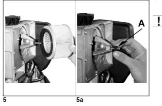
Clean the filtering element with air blast. Air must be blown from inside to outside the cartridge at a distance of at least 15 cm from the paper.
