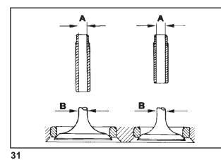
Dimensions and clearance between guides and valve stems (mm)
