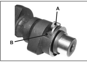
In case of a startup in reverse direction, the antireverse system lifts the valve as the tappet passes by. Startup is thus inhibited.
