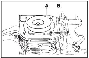
Lubricate the following parts with oil before mounting: the piston pin, the piston, the cylinder and the big-end bearing
