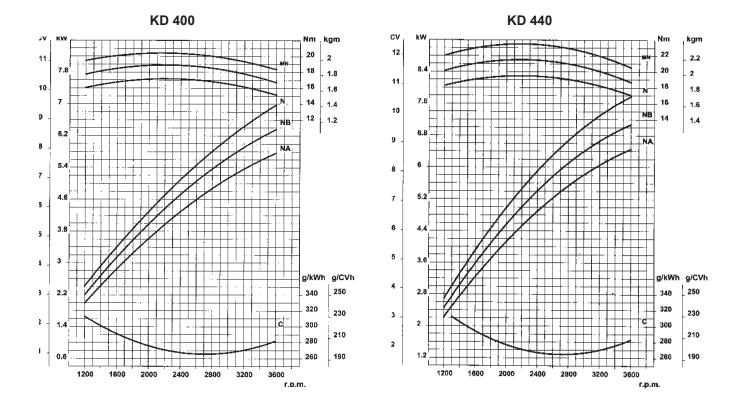
N (80/1269/EEC - ISO 1585) AUTOMOTIVE RATING : Intermittent operation with variable speed and variable load. NB (ISO 3046 - 1 IFN) RATING WITH NO OWERLOAD CAPABILITY: continuos ligth duty operation with constant speed and variable load. NA (ISO 3046 - 1 ICXN) CONTINUOS RATING WITH OVERLOAD CAPABILITY: continuos heavy duty with constant speed and constant load. MN Torque at N power.
