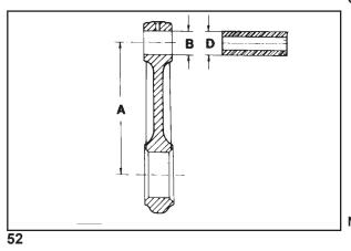
When remounting the big-end bearings, remember to thoroughly clean the parts and generously lubricate them to prevent seizure when the engine is started up for the first time
