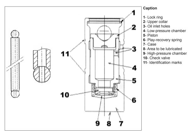
Fill the low-pressure chamber through the oil inlet holes.
