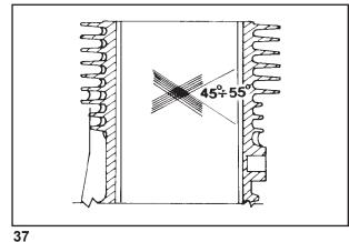
Do not manually hone the cylinder bore surfaces with emery cloth or other means.
