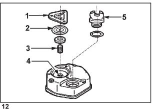
Always check the the spring and valve to make sure they are in a good conditions.
