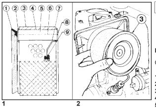
Clean the filtering element with air blast. Air must be blown from inside to outside the cartridge at a distance of at least 15 cm from the paper.
