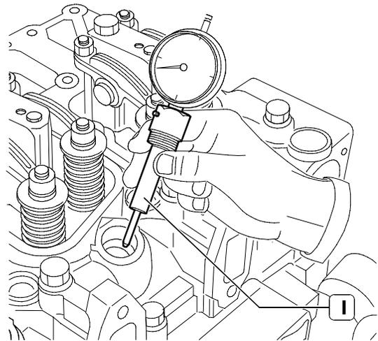
To find the top dead centre position of the cylinder, end of compression stage:
