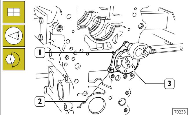
Set camshaft (3) retaining plate (1) with the slot facing the top of the engine block and the marking facing the operator, then tighten the screws (2) to the specified torque.
