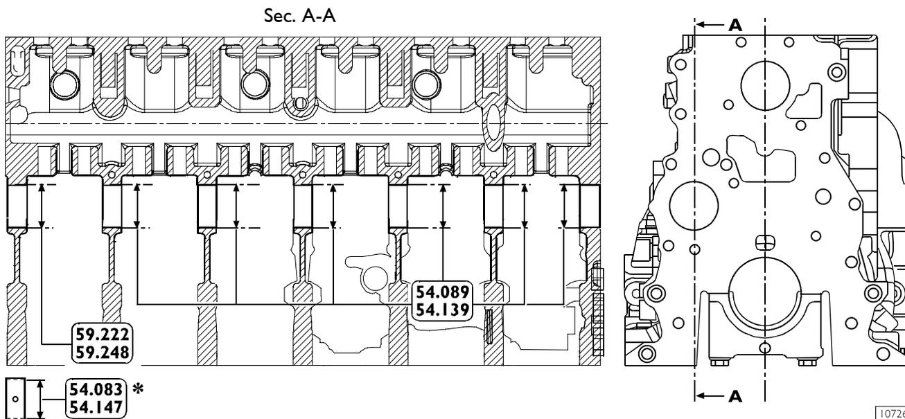
MAIN SPECIFICATIONS OF THE CAMSHAFT BEARING BUSH AND ITS SEAT (6-cylinder engines)
