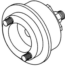
Tool for fitting output shaft rear gasket
