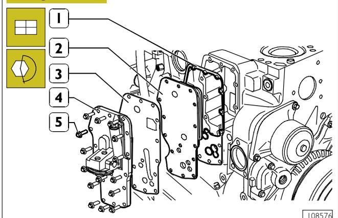
Fit on the engine block: a new gasket (1), the heat exchanger (2) a new gasket (3) and the oil filter support (4).
