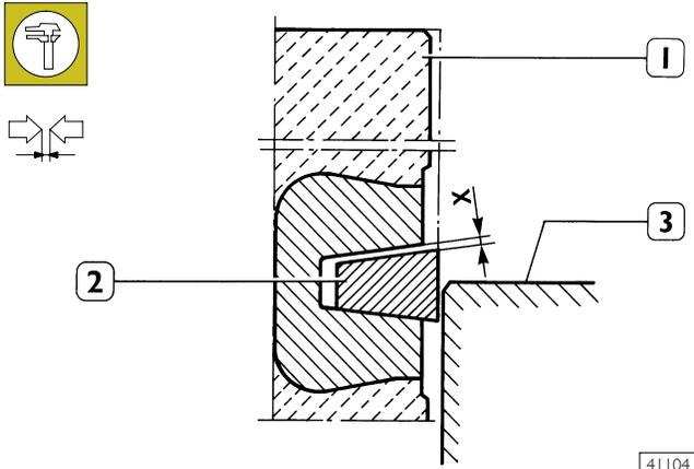
DIAGRAM FOR MEASURING THE CLEARANCE X BETWEEN THE FIRST PISTON SLOT AND THE TRAPEZOIDAL RING
