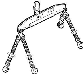
Lifting rig for engine removal/refitting
