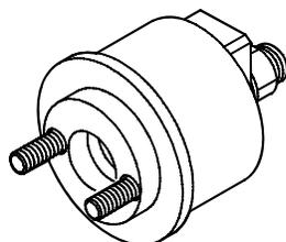
Tool for fitting output shaft front gasket
