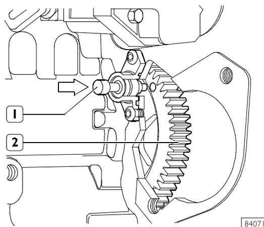
To find the position of cylinder n. 1 at top dead centre under full compression:
