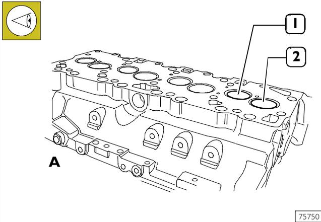
Intake (1) and exhaust (2) valves have heads with the same diameter.
