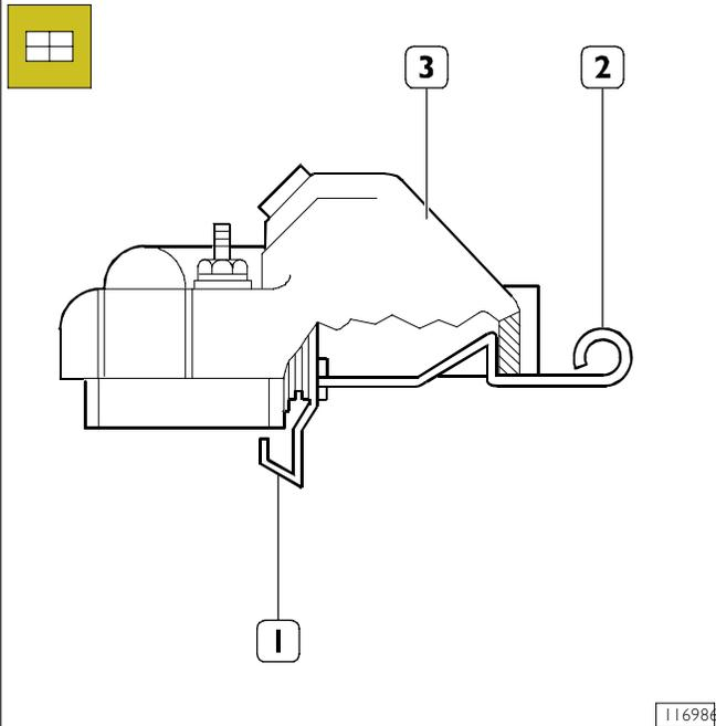
In the electro-valve ETR kit there is the joint tool (1) which must be used to position the electro-valve's arm (2) and to reassemble the cover on the injection pump.
