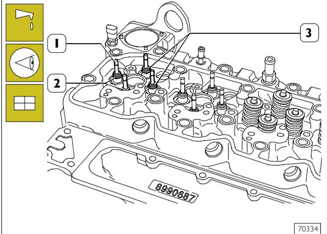
Lubricate the valve stems (1) and fit them into the relevant valve guides according to the position marked at removal.
