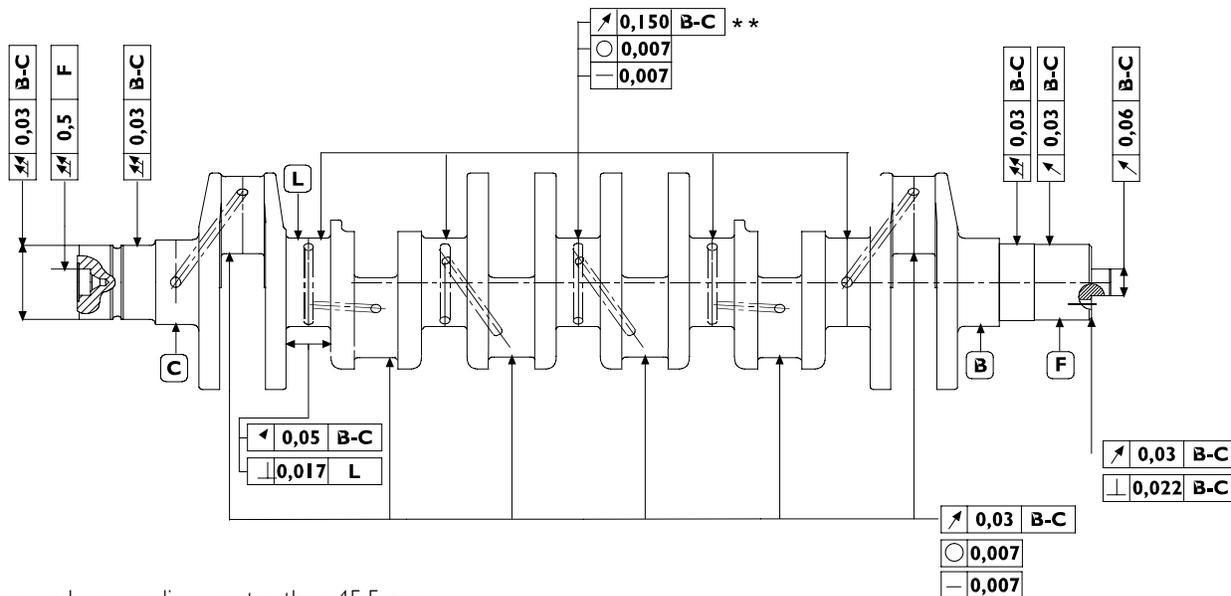
\* Measured on a radius greater than 45.5 mm
