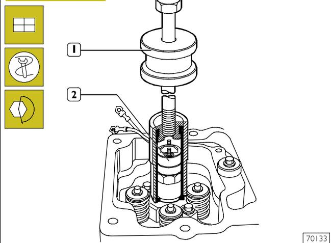
Use tool 99342101 (1) to fit the injector (2) into its seat. Screw injector fastening screws without tightening them.
