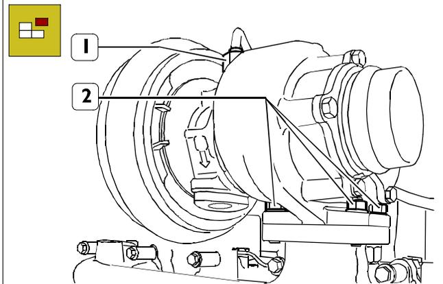
Proceed disassembling the supercharger:
