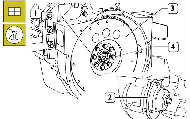
Apply tool 99360339 (2) to the flywheel housing to stop engine flywheel (3) rotation. Tighten the screws (1) fastening the engine flywheel (3) to the output shaft.
