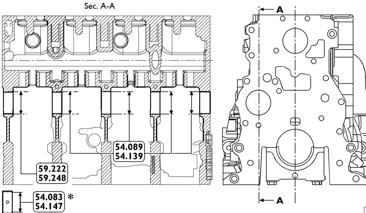
MAIN SPECIFICATIONS OF THE CAMSHAFT BEARING BUSH AND ITS SEAT (4-cylinder engines)
