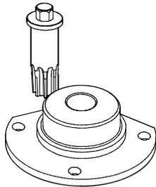
Tool for stopping the engine flywheel
