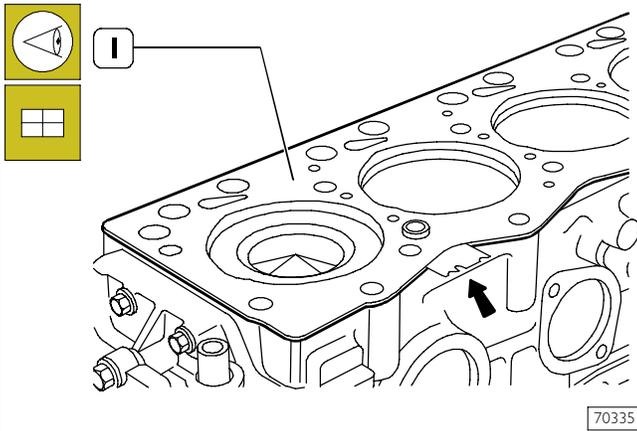
Check cleanness of cylinder head and engine block coupling surface.
