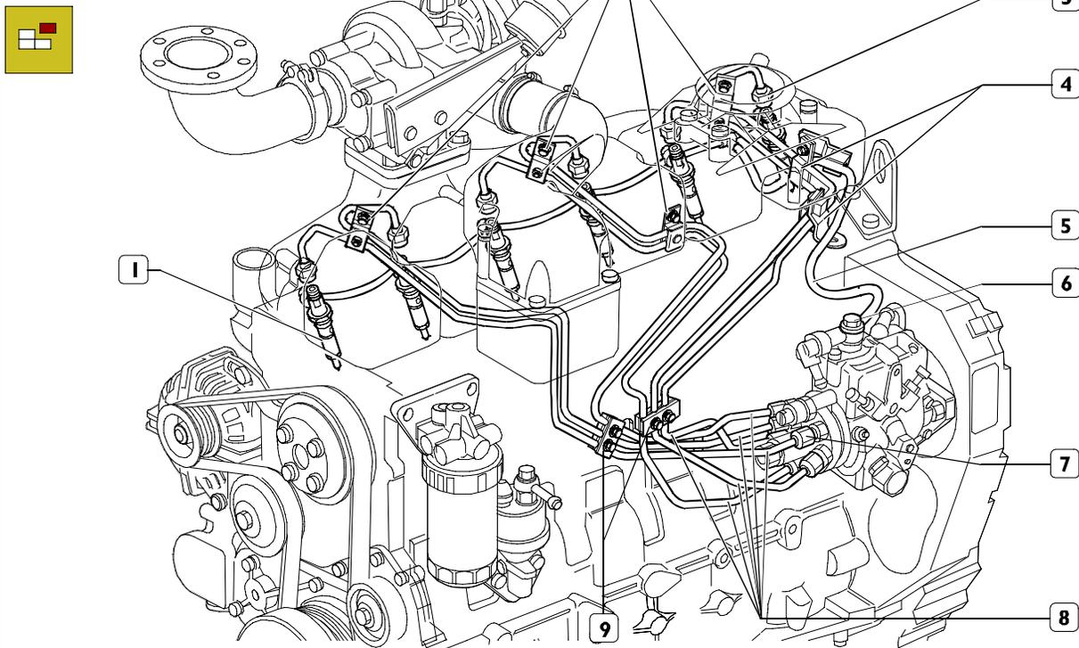
Remove the pipes forming the fuel supply (8) and recovery (5) between the pump and the injectors (1): unscrew the ring nuts (7) securing the pipes to the pumping elements; free the collar (6) of the fuel recovery pipe returning to the injection pump; undo the ring nuts (7) fitted on the injectors and unscrew the bolts securing
