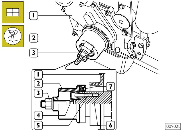
Apply tool 99346252 part (4) to the front output shaft tang (6), secure it by screws (5) and fit the new sealing ring (7). Position part (2) on part (4), screw nut (3) until completing sealing ring (7) fitting into front cover (1).
