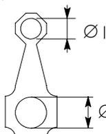
Ø 1 = housing for connecting rod small end bush
