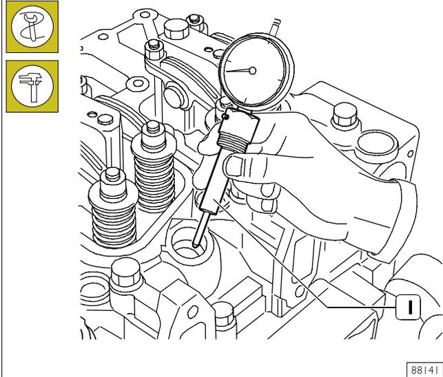
To find the top dead centre position of the cylinder, end of compression stage:
