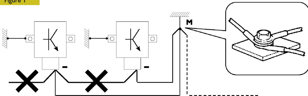
1. NEGATIVE CABLES "STAR" CONNECTION TO SYSTEM BONDING M
