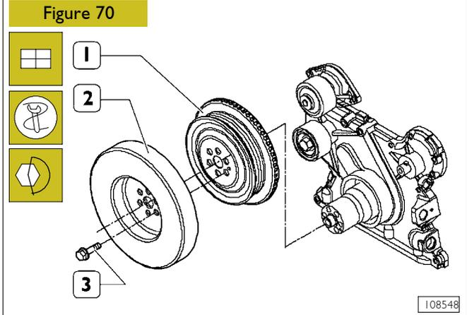
Assemble the pulley (1) and the damping flywheel (2) to the driving shaft.
