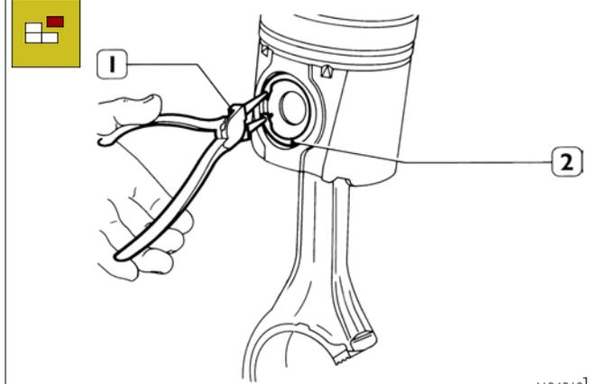
The circlips (2) retaining the gudgeon pin are removed using round-nose pliers (1).
