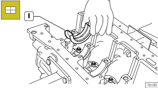
**NOTE** Refit the main bearings that have not been replaced, in the same position found at removal.
