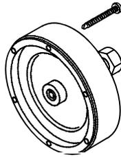
Tool to remove output shaft rear gasket
