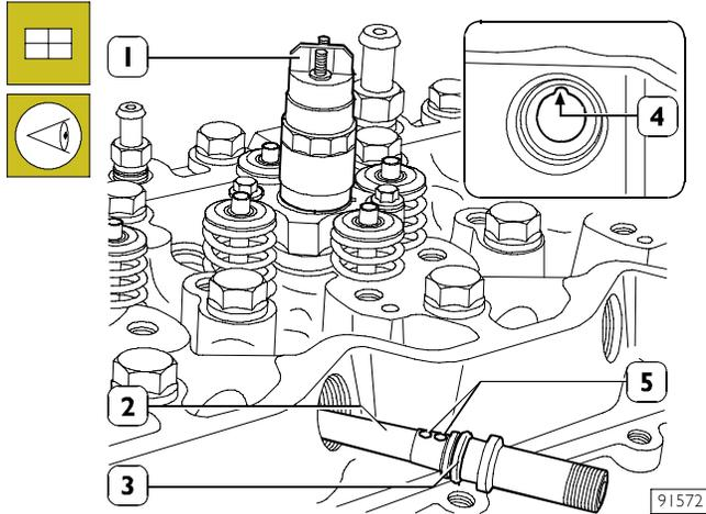
Fit a new sealing ring (3) lubricated with petroleum jelly on the fuel manifold (2) and fit it into the cylinder head seat so that the positioning ball (5) is coinciding with the relevant housing (4).
