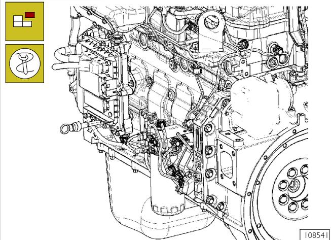
In order to apply the brackets 99361037 to the engine block to fix it on to the stand for the overhaul, it is necessary to perform the following operations on the left hand side of the engine:
