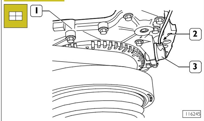
Fit a new sealing ring on the speed sensor (3).
