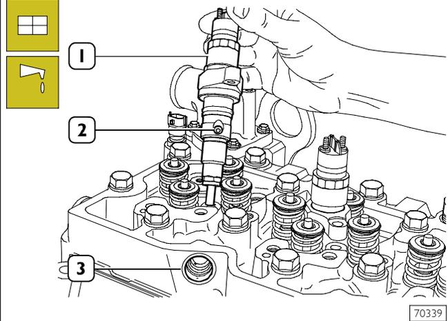
Fit injectors (1) on the cylinder head seats, directed so that the fuel inlet hole (2) is facing the fuel manifold seat (3) side.
