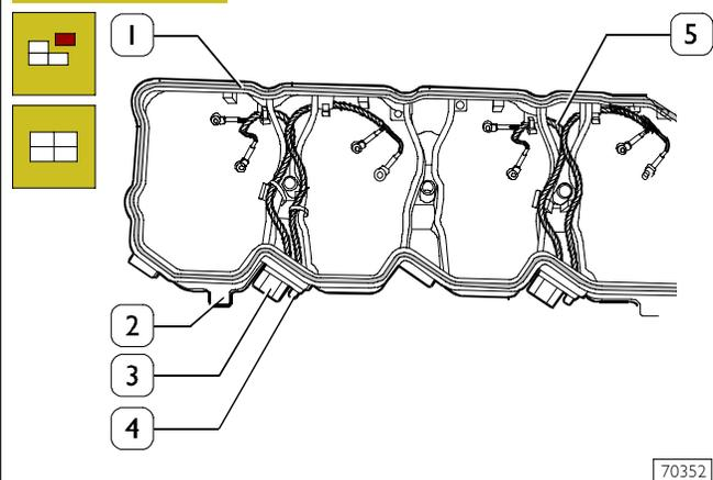
Check electrical cable (5) conditions, replace if damaged by cutting the support (2) clamps and removing the screws (4) that secure it to connections (3).
