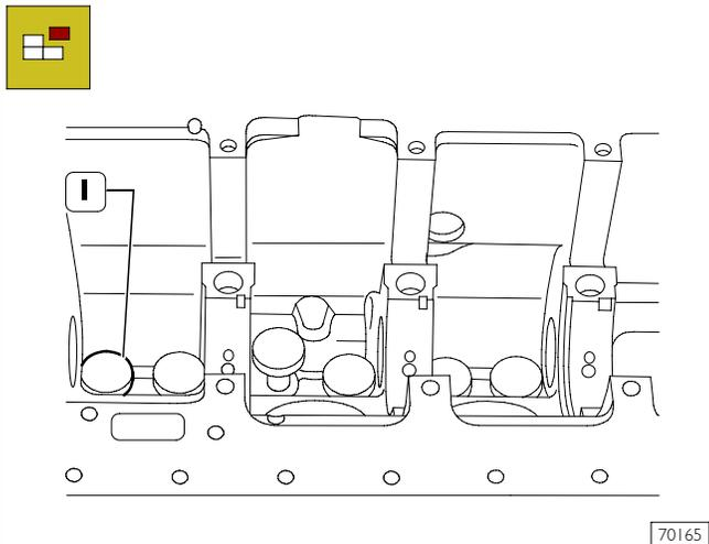
Withdraw the tappets (1) from the engine block.
