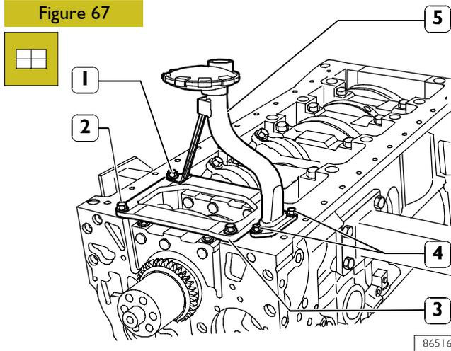
Fit the plate (3), the oil pick up tube (5) and tighten the fastening screws (1, 2, 4) to the specified torque.
