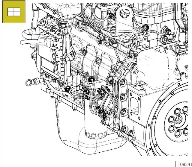
Assemble the bracket and the support of the fuel filter. Proceed connecting the pipelines (9,3,4 and 5) of the support to the high pressure pump.
