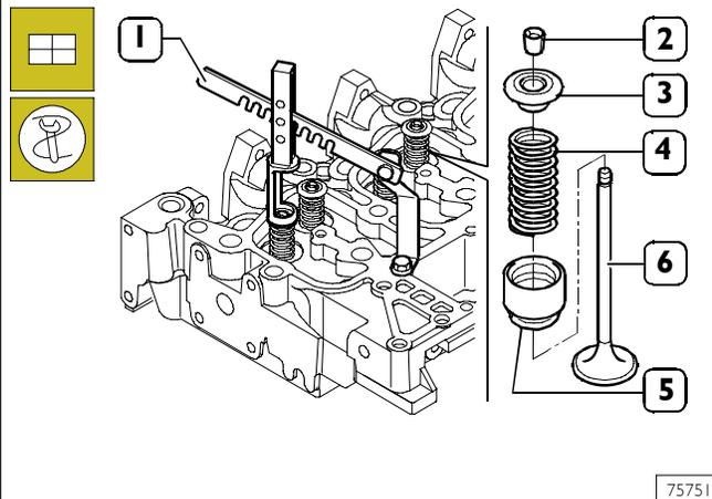
Position on the cylinder head: the spring (4), the upper cap (3); use tool 99360268 (1) to compress the spring (4) and lock the parts to the valve (5) by the cotters (2).
