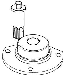
Tool for rotating/stopping the engine flywheel
