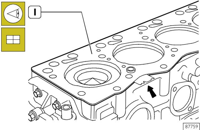
Check cleanness of cylinder head and engine block coupling surface.
