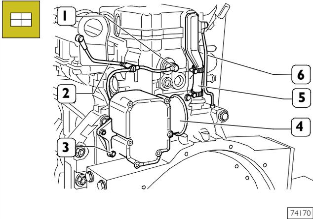
If present, insert blow-by filter (4) and tighten the screws (3).
