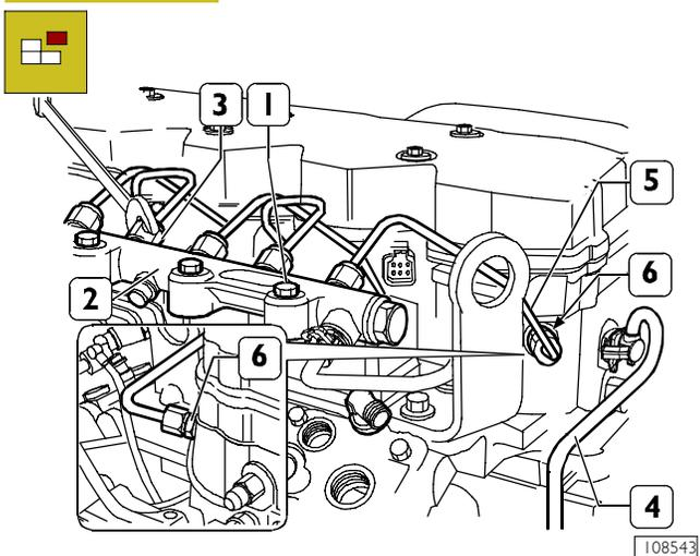
Disconnect from the rail (2): the fuel pipe (7) according to procedures described in Figure 15. Disconnect fuel pipes (5) from rail (2) and injector manifolds (6).
