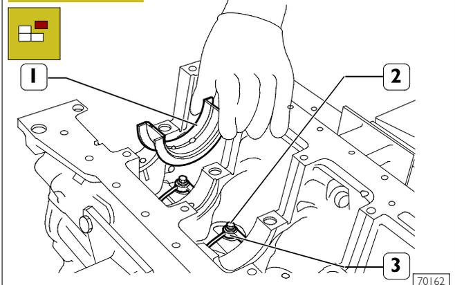
Remove the main half-bearings (1). Remove the screws (2) and remove the oil nozzles (3).
