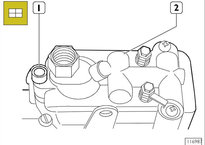
The repositioning of the cover (2) must be done proceeding in reverse to what described for its disassembling, making sure that it corresponds perfectly to the assembling seat without forcing it (for the ETR version the cover of the pump will correspond to the assembling seat only after the joint tool has been removed).
