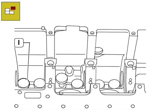
Withdraw the tappets (1) from the engine block.
