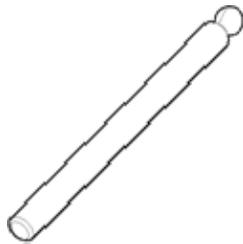
Tool for positioning of injection pump at start of discharge
