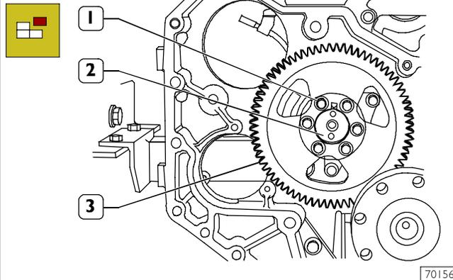
Remove the screws (1) and remove the gear (3) from the camshaft (2).
