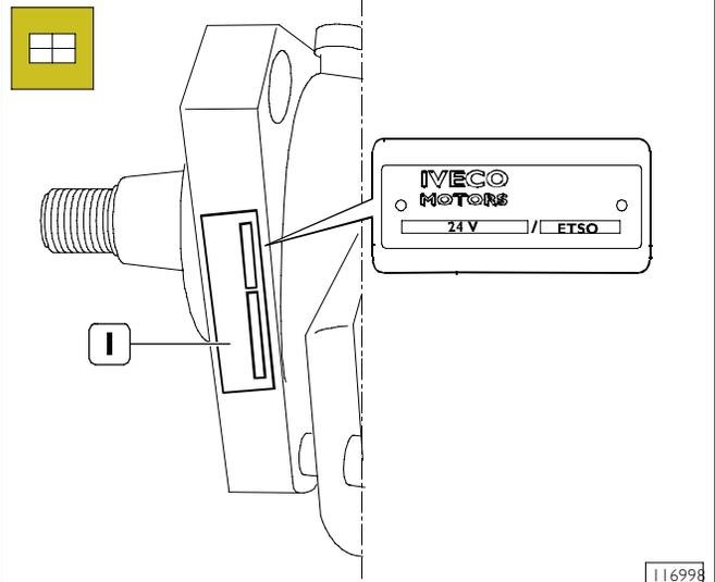
In case the original electro-valve should be replaced and its characteristics modified (different voltage, ETR instead of ETSO, eco), it is necessary the application of an identification tag (1) in the indicated place.
