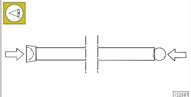
Rocker control rods shall not be distorted; the ball seats in touch with the rocker adjusting screw and with tappets (arrows) shall not show seizing or wear; otherwise replace them. Intake and exhaust valve control rods are identical and are therefore interchangeable.
