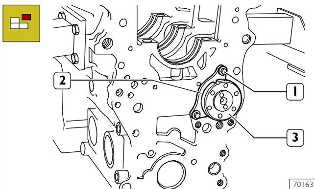
Remove the screws (1) and disconnect camshaft (3) retaining plate (2).
