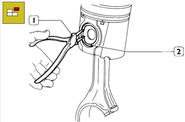
The circlips (2) retaining the gudgeon pin are removed using round-nose pliers (1).
