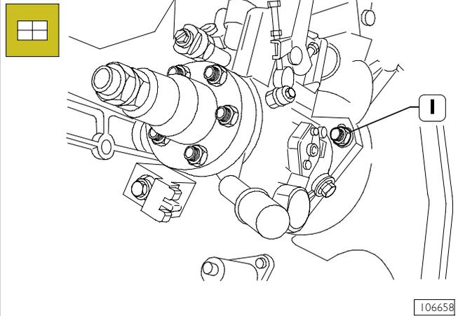
When installing supply pump on engine, cylinder no.1 must be at TDC, end of compression phase.
