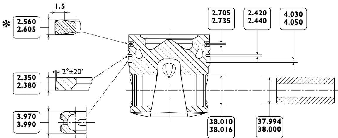
MAIN DATA OF THE PISTON WITH PIN TUNNEL AND PLASTIC RINGS
