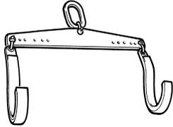
Tool for lifting the output shaft
