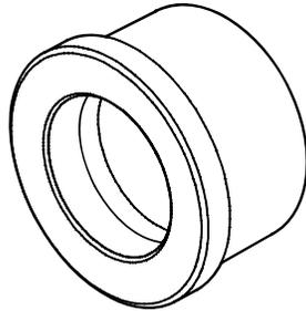
Beater for removing/refitting camshaft bushes (to be used with 993700069)
