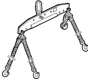
Lifting rig for engine removal/refitting
