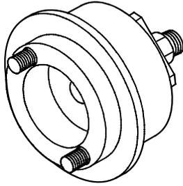
Tool for fitting output shaft rear gasket
