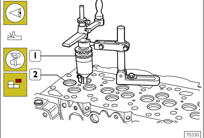
Should slight scratches or burns be found, go over with the adequate tool (1) according to the inclination values indicated in the Figure 69.
