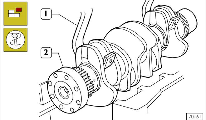
Use tool 99360500 (1) and hoist to remove the output shaft (2) from the block.
