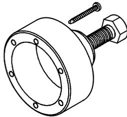
Tool to remove output shaft front gasket
