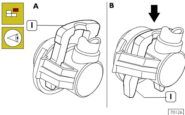
**NOTE** To disconnect fuel pipelines (3 and 4, Figure 26), in low pressure from the relating pipe fittings, it is Necessary to press the locking fastener (1) as shown in picture B.
