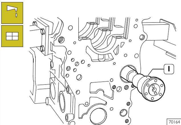
Lubricate the camshaft bush and fit the camshaft (1) taking care not to damage the bush or the housings.
