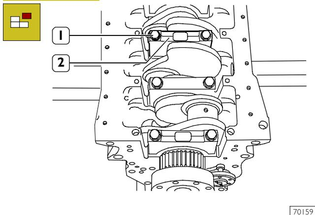
Remove the screws (1) and the main bearing caps (2).
