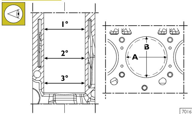
Measurements shall be performed on each cylinder, at three different heights in the barrel and on two planes perpendicular with each other: one parallel to the longitudinal axis of the engine (A), and the other perpendicular (B). Maximum wear is usually found on plane (B) in correspondence with the first measurement.
