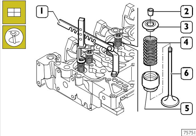
Valve removal shall be performed using tool 99360268 (1) and pressing the cap (3) so that when compressing the springs (4) the cotters (2) can be removed. Then remove the cap (3) and the springs (4).
