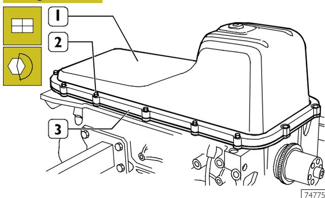
Fit the oil sump (1) and apply the plate (3) to it. Tighten the screws (2) to the specified torque.
