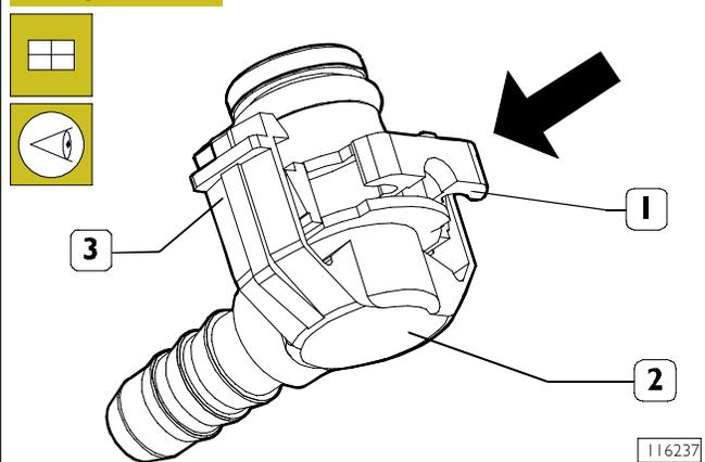
In order to connect the low-pressure fuel pipes to the connection joint, insert the rapid fitting joint into the latter, (2) and press until the clip fastens securely (3).
