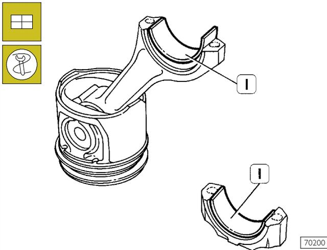
Fit half bearings (1) on connecting rod and cap.
