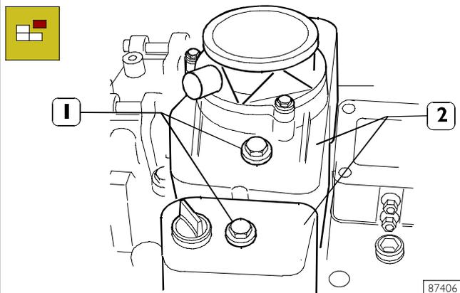
Remove tappet caps: Loosen the four fixing screws (1) and lift the caps (2); remove the gaskets.
