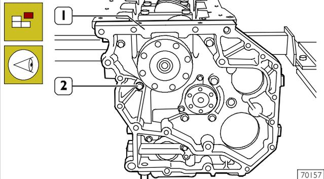
Remove the screws (2) and disconnect the timing gear case (1).
