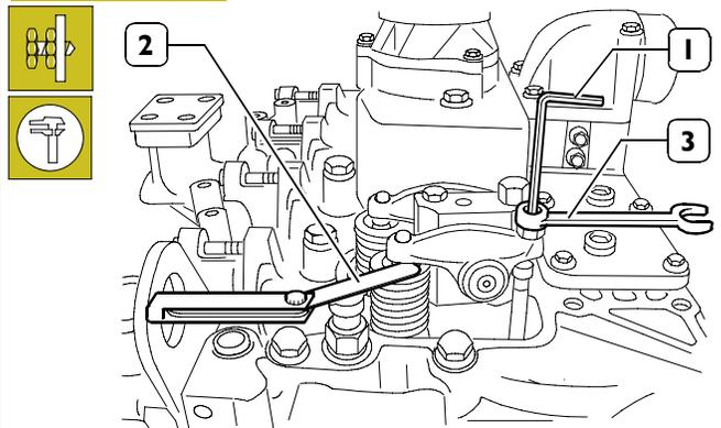
Adjust the play between the rocker arms and valves using a hex key (1), polygonal key (3) and feeler gauge (2).
