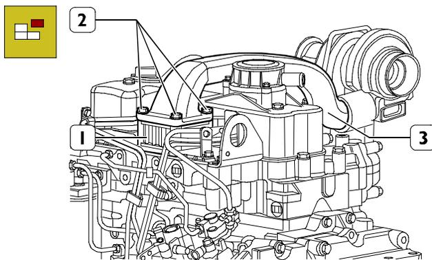
Loosen the screws (2), remove the duct (3) and the heater (1) (if present).
