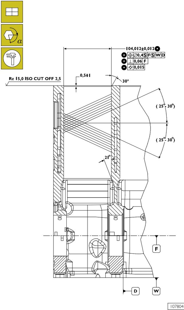
**NOTE** In case of regrinding, all barrels shall have the same oversize (0.4 mm).
