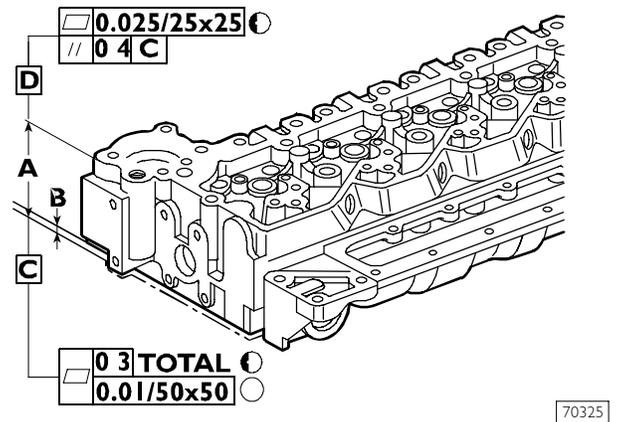
The rated thickness A for the cylinder head is  $105 \pm 0.25$  mm, max. metal removal shall not exceed thickness B by 1 mm.
