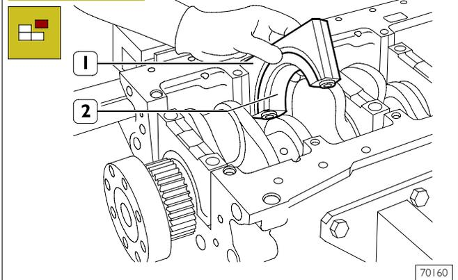
The second last main bearing cap (1) and the relevant support are fitted with shoulder half-bearing (2).
