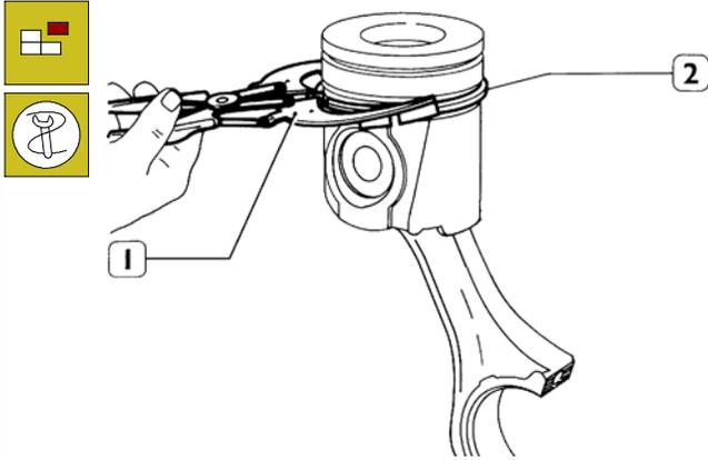
Remove split rings (2) from piston using pliers 99360183 (1).
