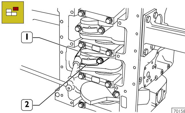
Remove the screws (1) fastening the connecting rod caps (2) and remove them.
