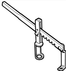
Tool for removing/refitting engine valves
