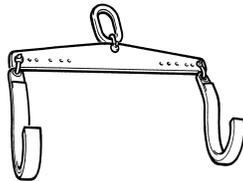
Tool for lifting the output shaft
