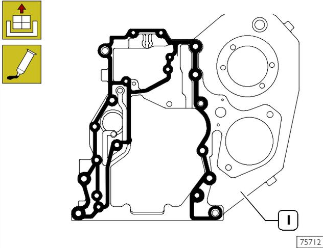
DIAGRAM SHOWING SEALING LOCTITE 5205 APPLICATION WITHIN GEARBOX AREAS
