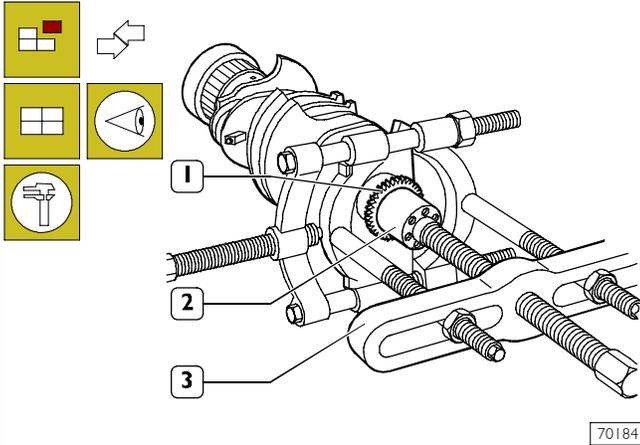
Check that gear tothing (1) is not damaged or worn, otherwise remove it using the proper puller (3).
