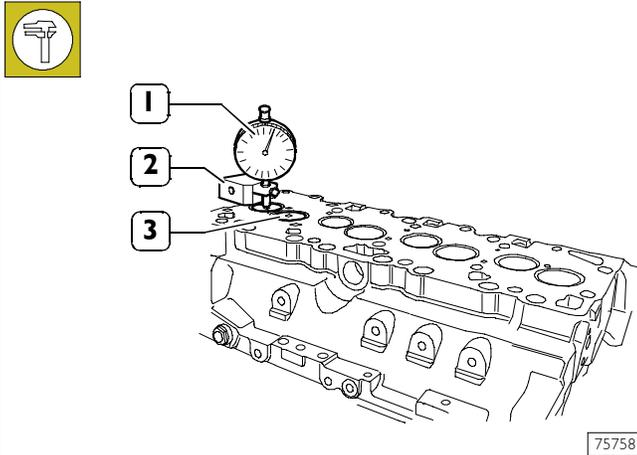
After regrinding, check that valve (3) sinking value is the specified one by using the base 99370415 (2) and the dial gauge 99395603 (1).
