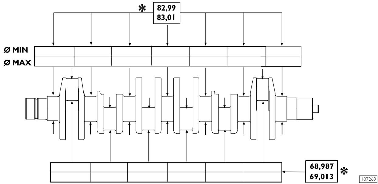
FILL THIS TABLE WITH OUTPUT SHAFT JOURNAL AND CRANKPIN MEASURED VALUES
