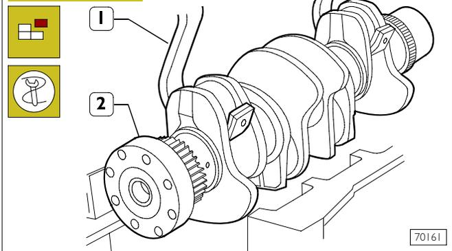
Use tool 99360500 (1) and hoist to remove the crankshaft (2) from the block.
