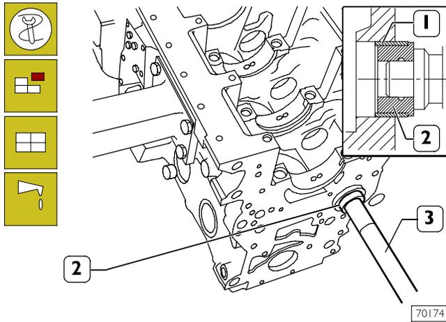
To replace the bearing (1) use tool 99360362 (2) and handle 99370006 (3) to remove and install it.
