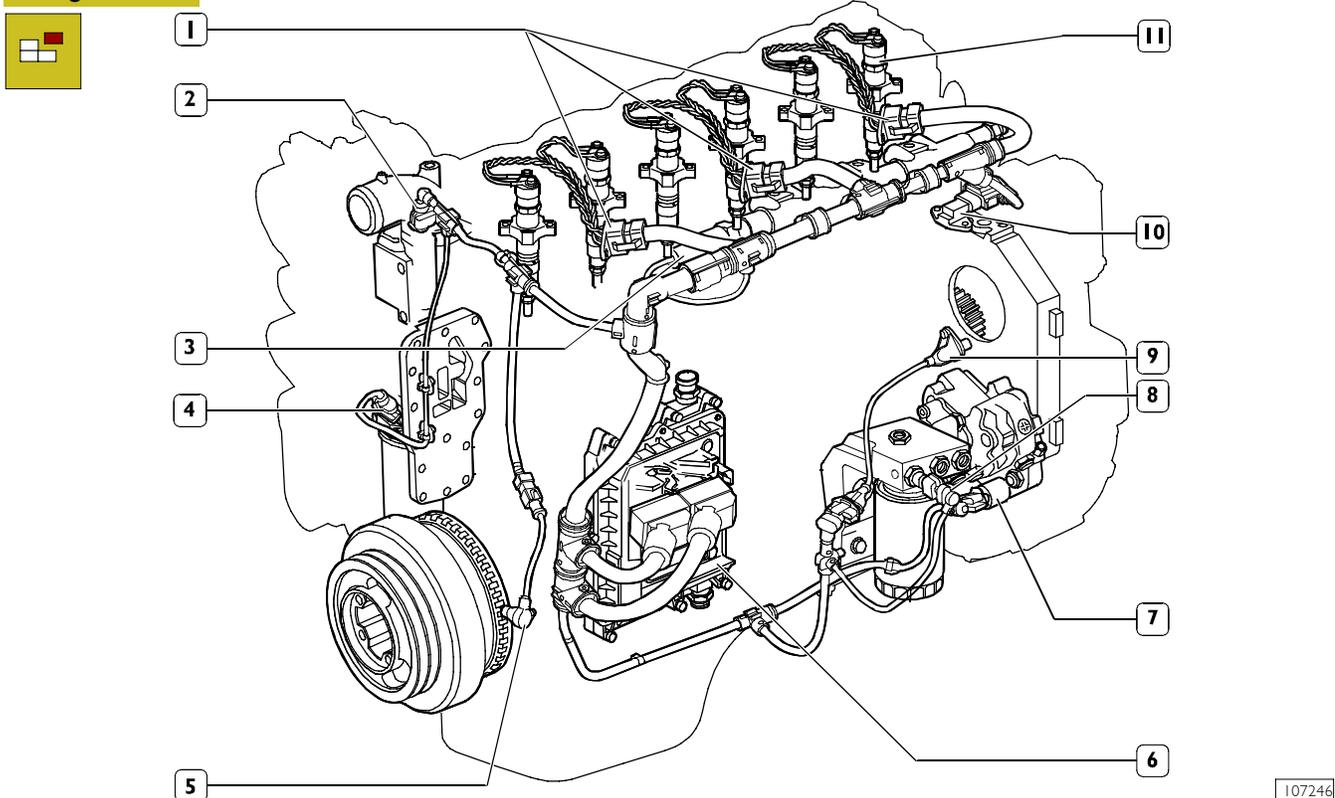
1. Connections for Electro-injectors - 2. Engine cooling liquid temperature's sensor - 3. Cable of the fuel pressure sensor - 4. Sensor of engine's oil temperature and pressure - 5. Driving shaft sensor - 6. EDC 7 gearbox - 7. Cable of pressure regulating gauge - 8. Cable of fuel heater and fuel temperature's sensor - 9. Timing system sensor - 10. Temperature - air pressure sensor - 11. Electro-injector.
