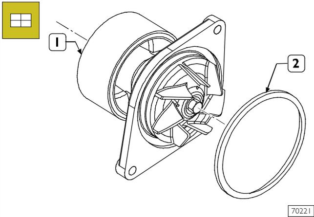
Apply a new sealing ring (2) to the water pump (1).
