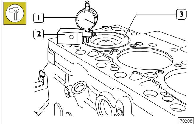
Once connecting rod-piston assemblies refitting is over, use dial gauge 99395603 (1) fitted with base 99370415 (2) to check piston (3) protrusion at T.D.C. with respect to the top of the engine block.
