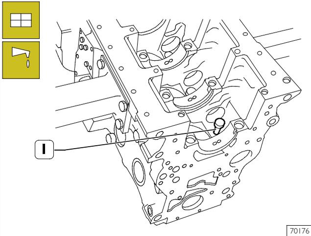
Lubricate the tappets (1) and fit them into the relevant housings on the engine block.
