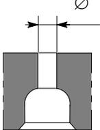
Valve guide seats on cylinder head                                | $\varnothing 1$                                                                                                                                                                                                                    | mm<br>8.019 to 8.039                               |
