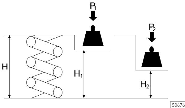
**MAIN DATA TO CHECK INTAKE AND EXHAUST VALVE SPRINGS**
