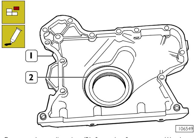
Remove the sealing ring (2) from the front cover (1), clean accurately the coupling surfaces and smear them with LOCTITE 5205.
