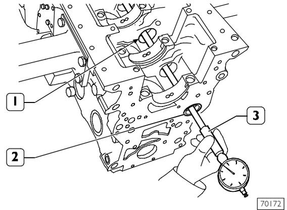
Camshaft bushes (2) shall be pressed into their housings. Internal surfaces must not show seizing or wear. Use bore dial gauge (3) to measure camshaft front and rear bush (2) and intermediate housing (1) diameter. Measurements shall be performed on two perpendicular axes.
