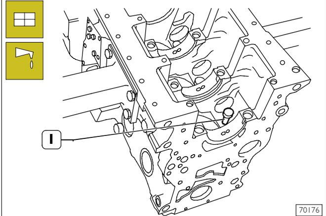
Lubricate the tappets (1) and fit them into the relevant housings on the engine block.
