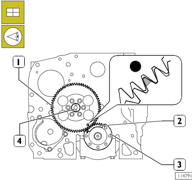
Turn the engine shaft (3) and the distribution shaft (4) so that by mounting the bevel gear on the latter (1) the stencilled mark on the gear (1) coincides with the groove on the gear tooth (2).
