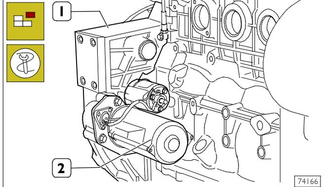
Remove the starter (2) from the flywheel housing (1).
