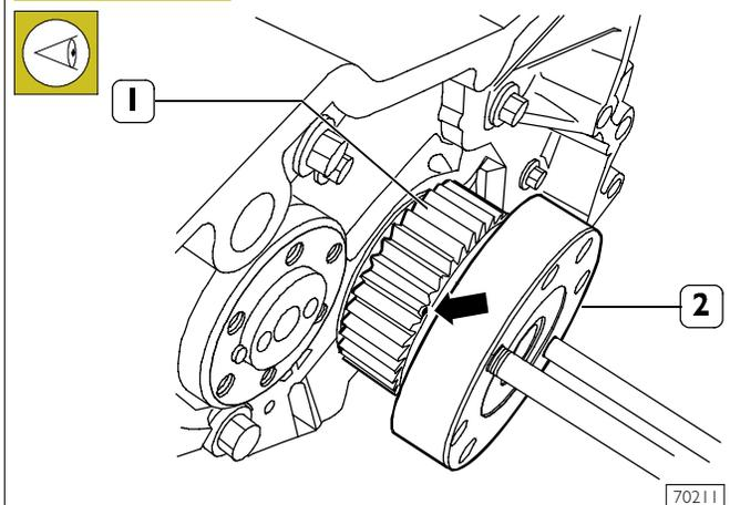
With a felt-tip pen, highlight the conducting gear tooth (1) mounted on the engine shaft (2) upon the side surface of which a groove has been created for the ignition timing.
