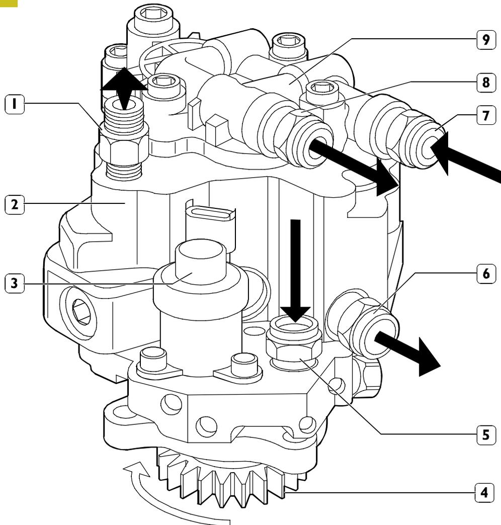
1. Fuel exhaust connector to rail - 2. High pressure pump - 3. Pressure regulating gauge - 4. Driving gear - 5. Connector to fuel entry flowing from filter - 6. Connector to fuel exhaust to filter support - 7. Connector to fuel entry flowing from engine control module heat exchanger - 8. Connector to fuel exhaust flowing from mechanic pump to filter support - 9. Mechanical feeding pump.
