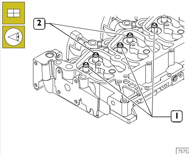
Remove the seals (1 and 2) from the valve guides.
