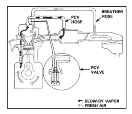
The Positive Crankcase Ventilation (PCV) system recirculates the crankcase blow-by gases into the intake manifold to be combusted in the engine. When the blow-by vapor pressure is high enough to overcome the spring pressure in the PCV valve, the valve opens to allow blow-by vapor into the intake manifold for combustion along with the fuel/air mixture.
