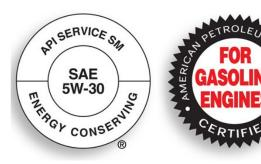
PSI recommends using engine oils that have an API rating of SM or newer. Gasoline engines that are converted for LPG or NG fuels MUST use oils labeled 'FOR GASOLINE ENGINES'. Do not use oils that are specifically formulated for Diesel Engines only. CC or CD classifications oils, even when labeled Heavy Duty or for Natural Gas Engines, **ARE NOT ACCEPTABLE.**
