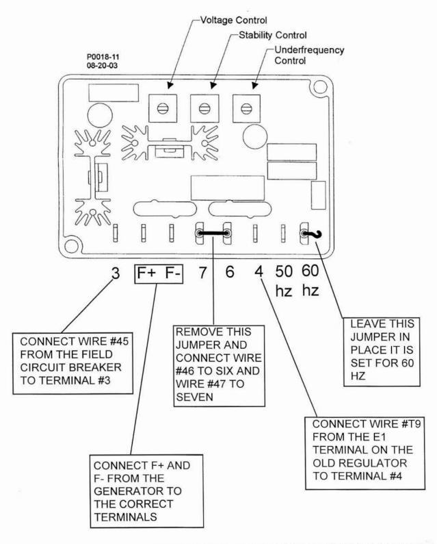
ALL OTHER WIRES ARE JUST CAPED OFF. IF YOU HAVE MORE THAN ONE LEAD ON A TERMINAL THEY MUST BE MOVE TOGETHER OR CAPPED TOGETHER
